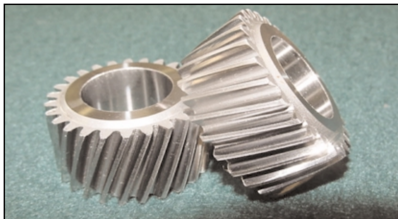
Figure 4—Photograph of helical gear pressed in the collaborative effort. Note gear has a 22° helix angle with an OAL of 22.5 mm. The major diameter of the gear is 42.5 mm and the ID of the gear is 23.5 mm.
