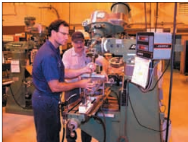
A setup reduction event resulted in a new fixture and quick-change tooling on this Bridgeport milling machine at Triumph Gear Systems.
