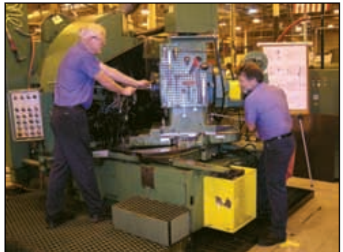
At Triumph Gear Systems, standardized work allows more than one operator to participate in changeovers. Also, keeping tools close at hand eliminates wasted steps.
