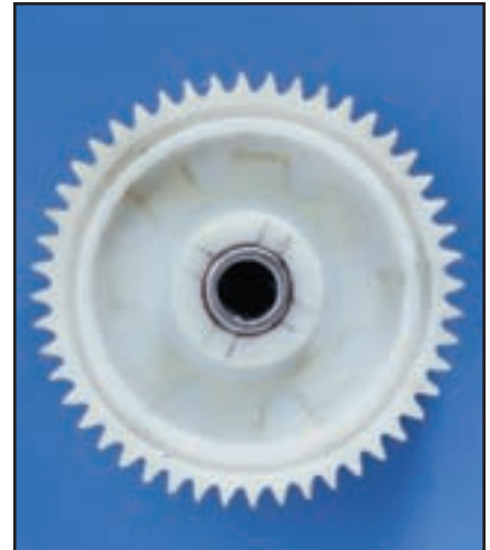
Figure 5—Thinned gear teeth.
