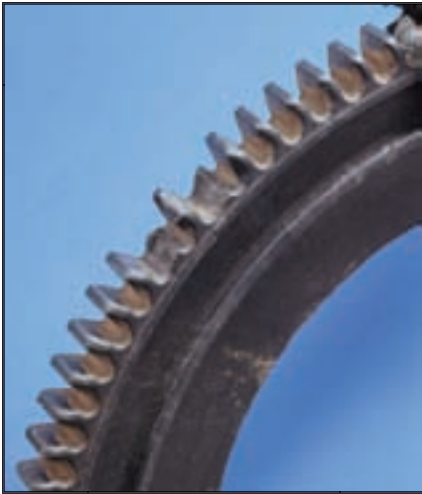
Figure 3—Gear with broken teeth.
