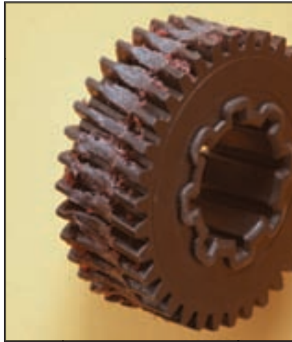
Figure 4—Gear with melted teeth.
