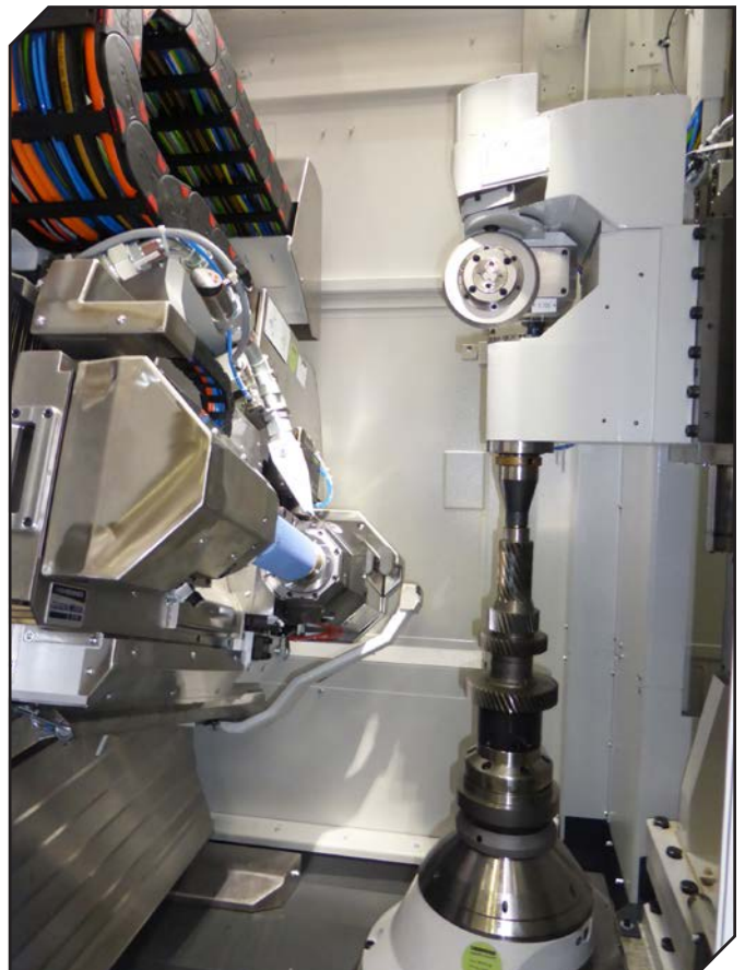
The trend for a finer surface roughness will lead to use finer grain sizes in the finishing cut, according to Andreas Mehr, Liebherr grinding and shaping technology developer.
