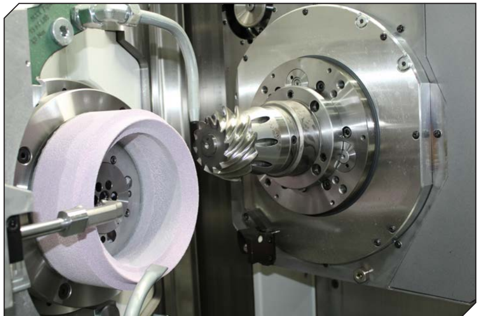
Xtrium bevel gear grinding wheel from Norton | Saint-Gobain.
