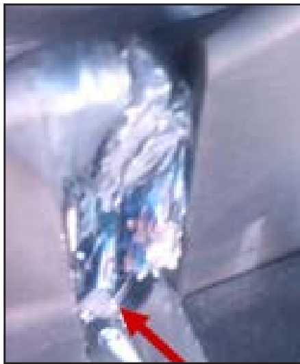
Figure 5 Chip packing between two blades.
