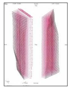
Figure 2 Topography measured on a single tooth combining a single helix 2-D line scan on each flank with multiple profile 2-D line scans.
