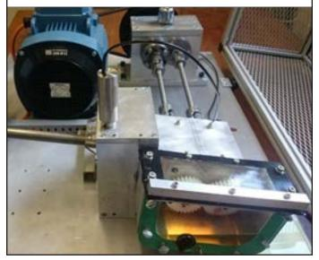
(b) Oil lubricated conditions Figure 1 Two gear test rigs.
