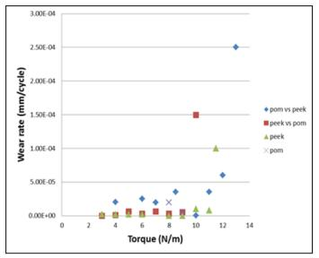
Figure 8 Wear rate against load for POM and PEEK gears.
