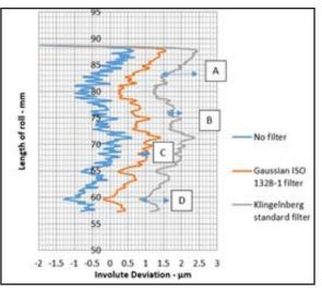
Figure 5 Profile results with different filters (Sample 1).
