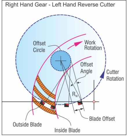
Figure 6 Face hobbing, right-hand gear with left-hand reverse cutter head.
