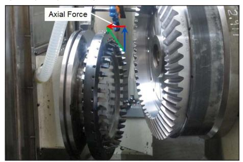
Figure 2 Left-hand gear cut with right-hand cutter.
