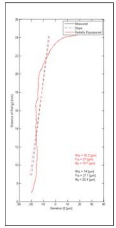
Figure 3 Change in profile parameters with data spacing strategy for large deviations with 480 data points.
