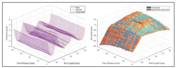
Figure 7 Residual form deviation after extraction of the surface polynomial and a comparison of the synthesized surface with the measured surface.
