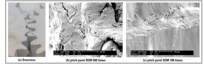
Figure 3 Experimental results for polycarbonate gears.
