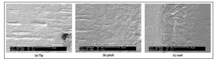
Figure 7 PA gear tooth SEM results.
