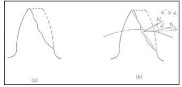
Figure 9 Typical wear form for POM gears (Ref. 2).
