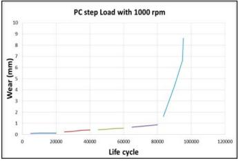
Figure 2 Experimental results for polycarbonate gears.
