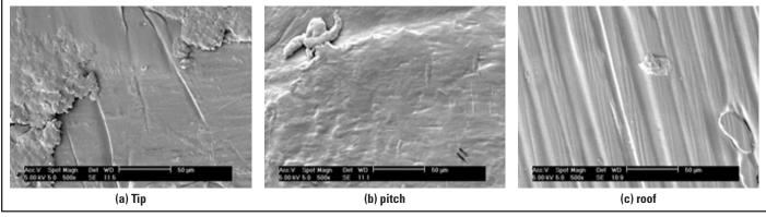
Figure 6 PEEK gear tooth SEM results.
