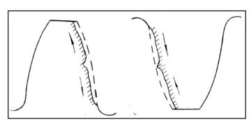
Figure 4 Gear surface wear (Ref. 2).
