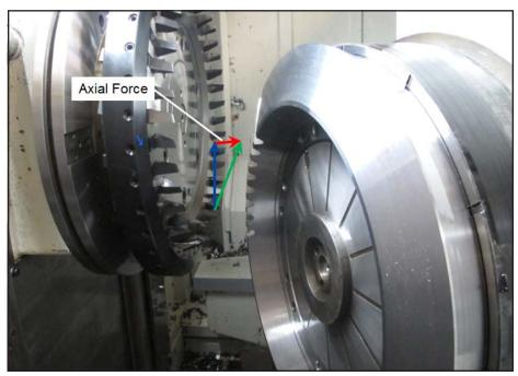
Figure 1 Right-hand gear cut with right-hand cutter.
