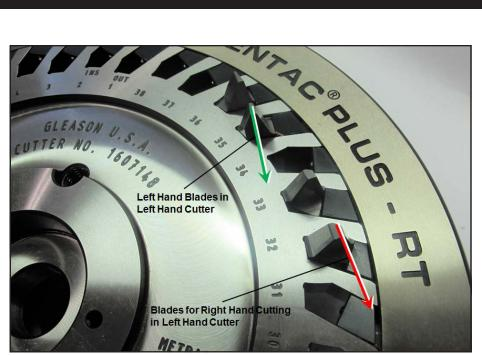
Figure 7 Standard blades for LH cutter and special blades for RH gear.
