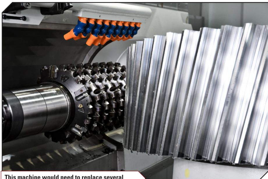
This machine would need to replace several planing machines and be able to manufacture spur, helical, double helical, or herringbone gears.
