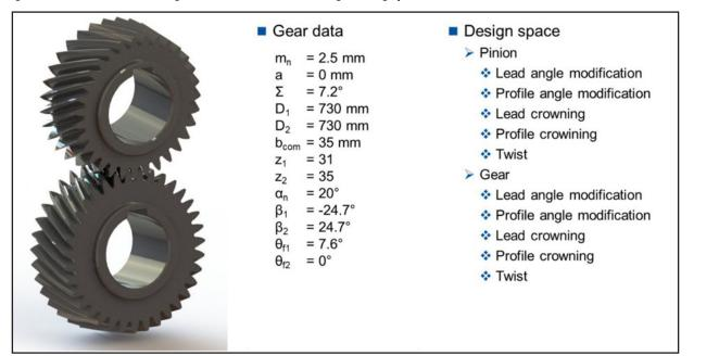
Figure 4 Gear data of test gear set and design space.
