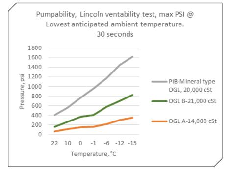
Figure 6 Residual pressure at lowest testing temperature.
