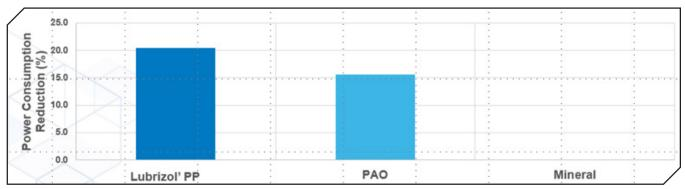
Figure 10 Lubrizol OGL with PP technology shows better performance in energy consumption in FZG rig.
