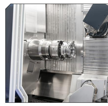
up the tools parallel to machining time and to automatically access the stock in the magazine. Stored tools can therefore be placed in the upper and lower tool holder. With the integrated loading concept, WFL has reduced the space requirement by 50% in comparison to a conventional produc-tion cell.
