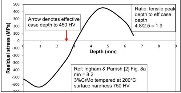
Figure 2 Induction-hardened residual stress profile (Ref. 2).
