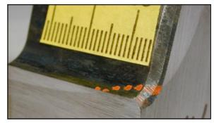
Figure 5 Unhardened area at end of tooth.
