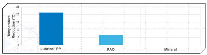
Figure 8 Lubrizol OGLs with PP technology shows better performance in temperature reduction in FZG rig.
