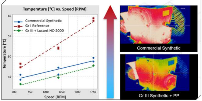
Figure 4 Gr III Synthetic with PP vs. PAO Synthetic.
