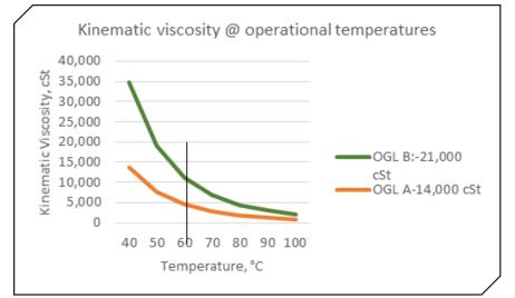
Figure 5 Viscosity of Lubrizol's OGLs with PP technology at different temperatures.
