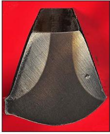
Figure 1 Bending fatigue failure of inductionhardened gear.
