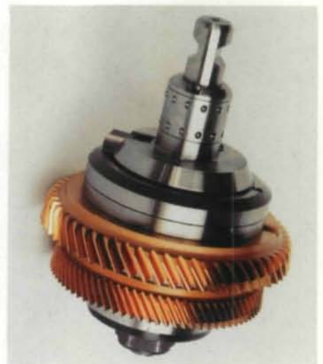
Fig. 12B—Cutter adapter with ball cage for concentric location of cutter to cutter spindle.
