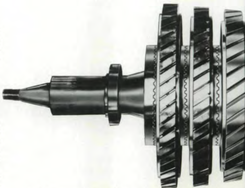
Fig. 2—A compressor rotor assembly for an aircraft jet engine. The Fixed Curvic Coupling is used to accurately position the separate interchangeable discs.
