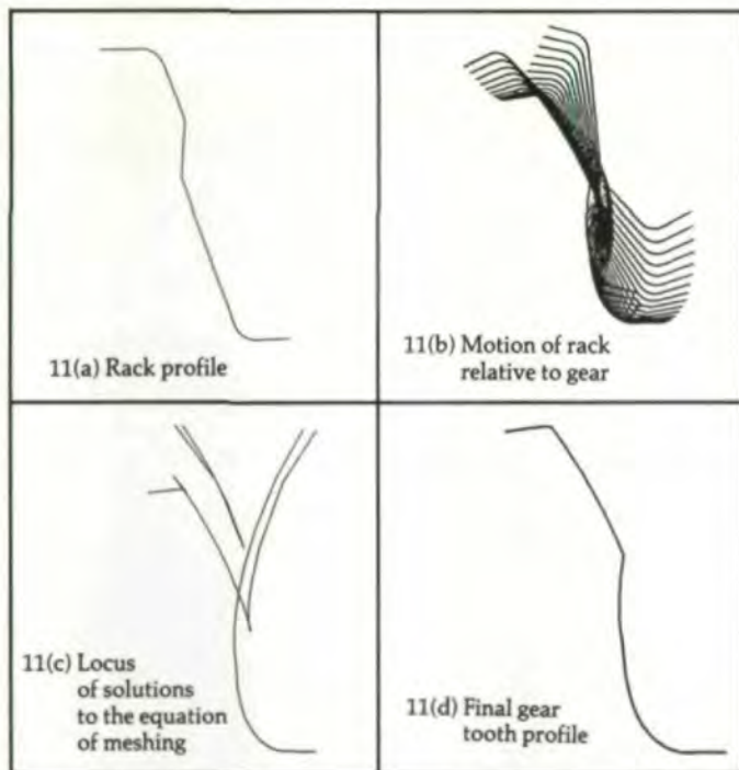
Fig. 11 - Generation of a gear using a rack with a protuberance angle \alpha = 25^\circ .
