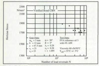
Fig. 6 — Endurable Hertzian face stress  $\sigma_{\rm H}$  of case hardened gears (newly dressed vitrified bond CBN wheel, Variant 46).
