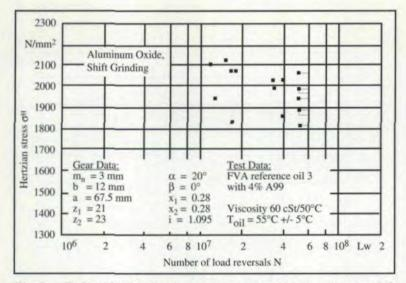
Fig. 5 — Endurable Hertzian face stress  $\sigma_{\rm H}$  of case hardened gears (shift grinding aluminum oxide, Variant 111).
