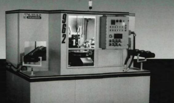
Over two years of intense development has been spent on the revolutionary **962 ADS System**. New Technology (Pat. Pend.) has been developed to allow precision high volume deburring automatically. No operator is needed except to replenish the tool reservoir after approximately 26,000 parts have been deburred. Reloading tool system takes only a few minutes. Computer controls feature a self diagnostic system, a part process monitoring and CIM communications.
