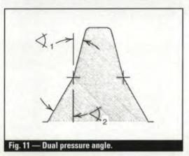
tapered. Gears cut by a hob with flute lead error will not have the correct involute form. The teeth are unsymmetrical, each side of the teeth having a different pressure angle. The teeth are said to be "leaning" or have cross bearing. The leaning of the teeth can be seen in the involute diagram (Figs. 8-9).
