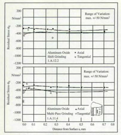
Fig. 1 — Residual stress pattern in the surface zone of the variants shift grinding aluminum oxide (Variant 12) and multi-pass grinding aluminum oxide (Variant 11).
