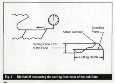
**Rake angle error.** The hob cutting face is designed to lie in a specified plane, and any variations of the actual hob flute cutting face from that plane are considered flute cutting face error. This error is measured from the outside diameter to the cutting depth. (See Fig. 1).
