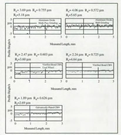
Fig. 4 — Recordings of roughness measurement of the ground surface of the tested gear variants in the initial state.
