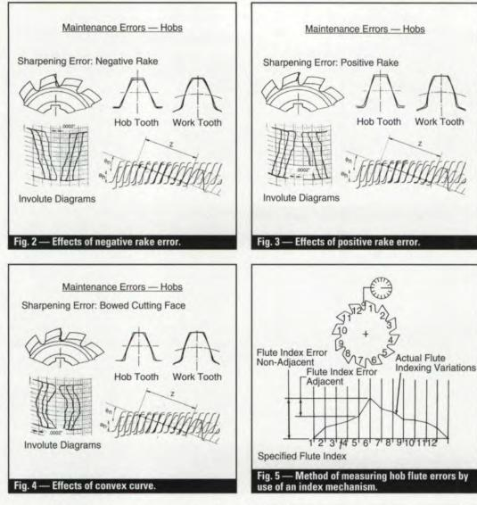
flutes will not produce the correct involute form. The hob will have high and low teeth which will produce unequal generating flats on the gear teeth. High hob teeth will produce low flats or hollows on the gear profile. The resulting involute diagram will be wavy due to the high and low spots on the profile.
