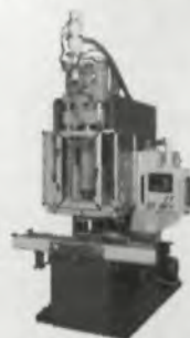
WPC50/1500 C-frame injection machine
