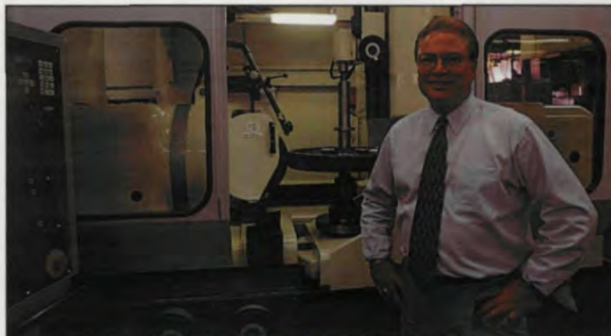
Fig. 1 – Joe Gelles, president of Acme gear, with the modified Reishauer RZ820 used to grind centrifugal compressor gears.
