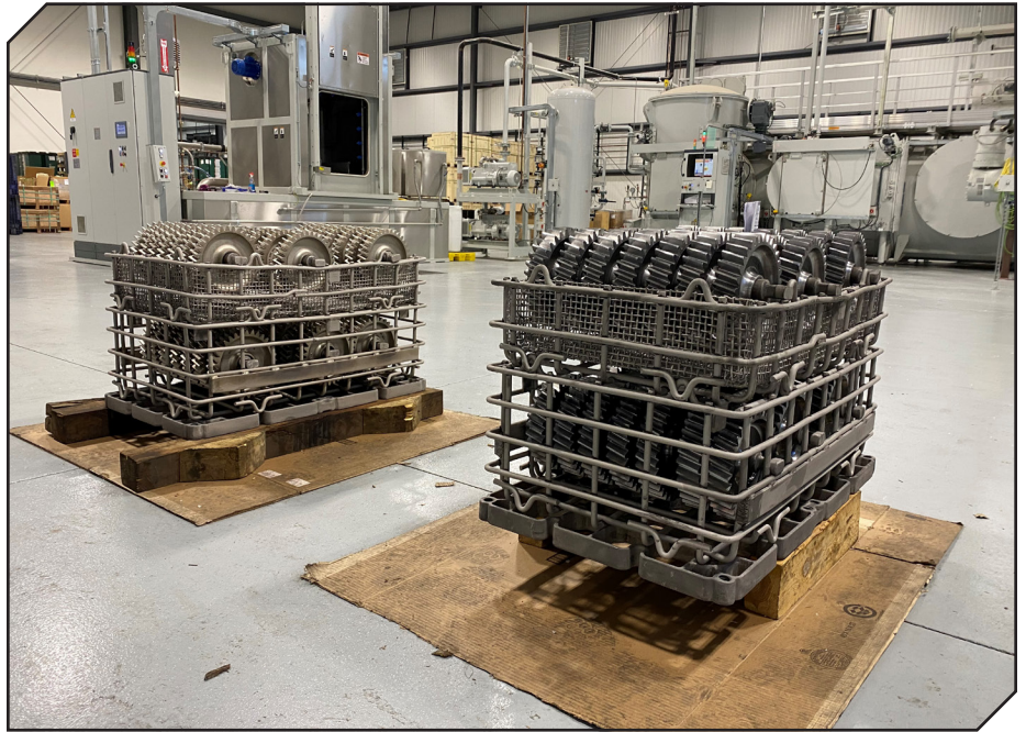
Large gears necessitate oil quench (all photos courtesy of Nitrex).
