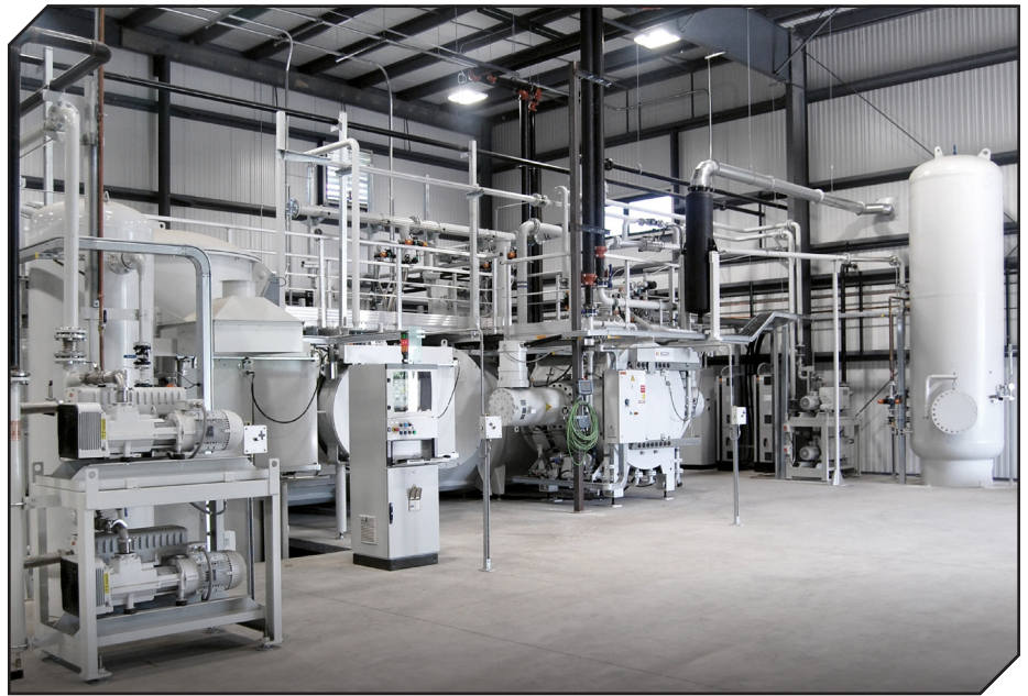
Modern high production low pressure carburizing furnaces at Nitrex HTS – Aurora, IL.
