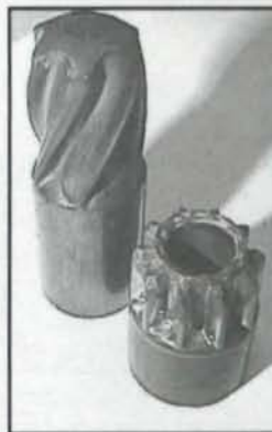
Figure 3—Extrusion-forged gear forms.
