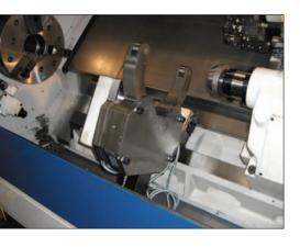
The LZ90-360 offers a clamping range with a minimum of 90 mm and a maximum 360 mm, the LZ150-420 from 150 mm to 429 mm and the LZ110-500 has a range from 100 mm to 500 mm.
