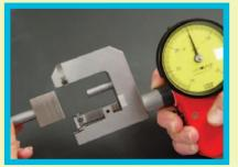
Internal or External Spline Measurement Made Easy!
