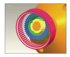
Rolled out at EMO 2007, the Scudding process is a continuous cutting operation that uses a tool design similar to a helical shaper cutter. It can be used for a wide range of gear applications including involute gears like sprocket or ring gears or on non-involute or non-symmetrical gears, like belt pulleys or straight synchronic gears.
