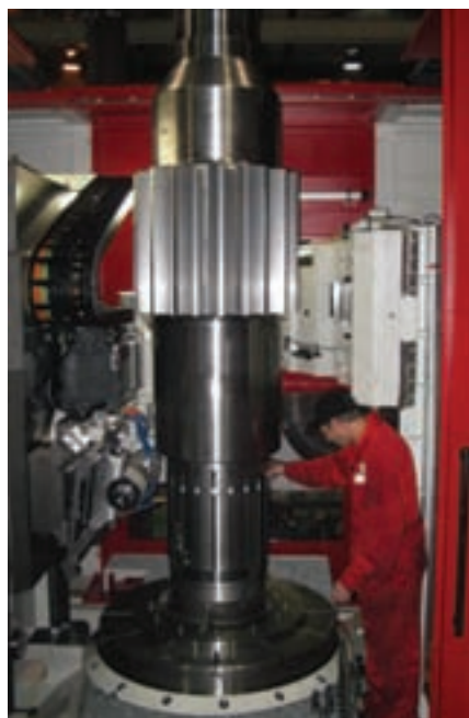
Large gears also require large pinions. Photo/Vancouver Gear Works.
