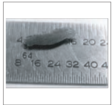
Figure 2—Debris found on chip detector.
