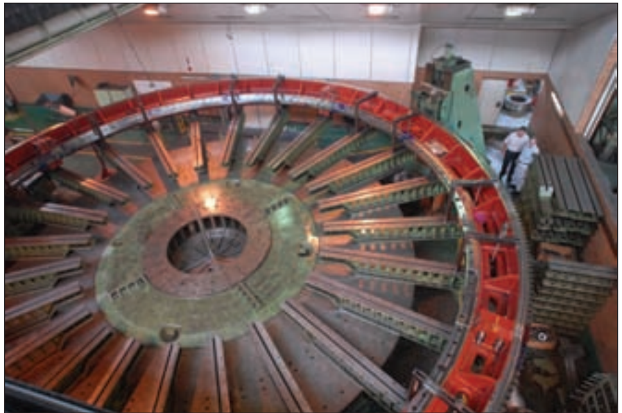
David Brown engineers inspect the 12.4 m diameter girth gear under construction at the Benoni plant in South Africa.
