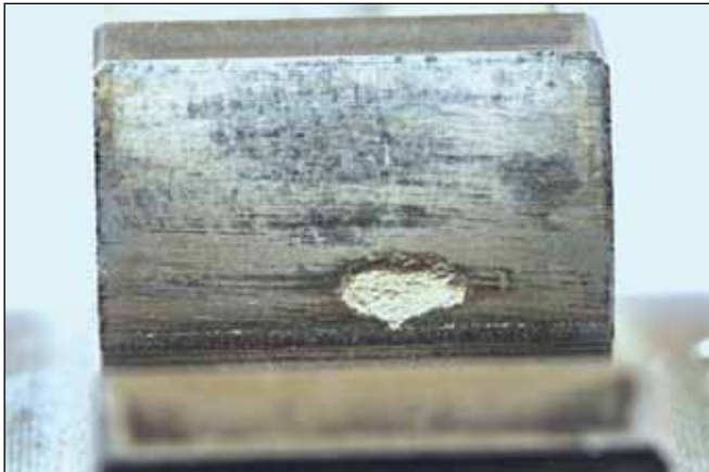
Figure 5—Damage caused by tip-to-root interference on pinion.
