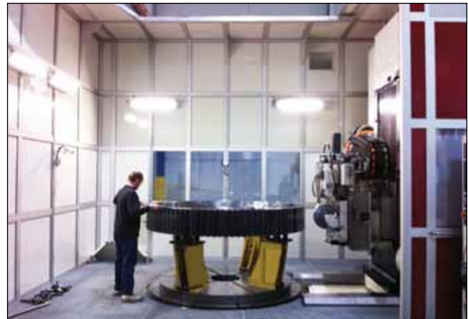
The ZP 40 is capable of grinding 4,000 mm diameter and 1,750 mm face width gears.
