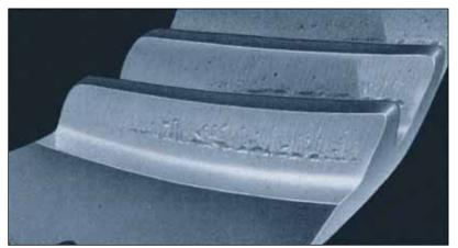
Figure 7—Pitch-line pitting on a spiral bevel gear surface.
