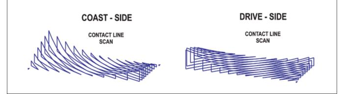
Figure 3—Contact-line scan of a spiral bevel gear set.
