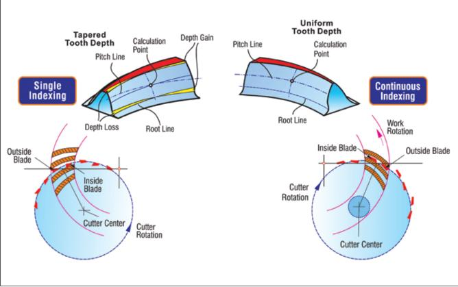
Figure 5—Left: face milling; Right: face hobbing.
