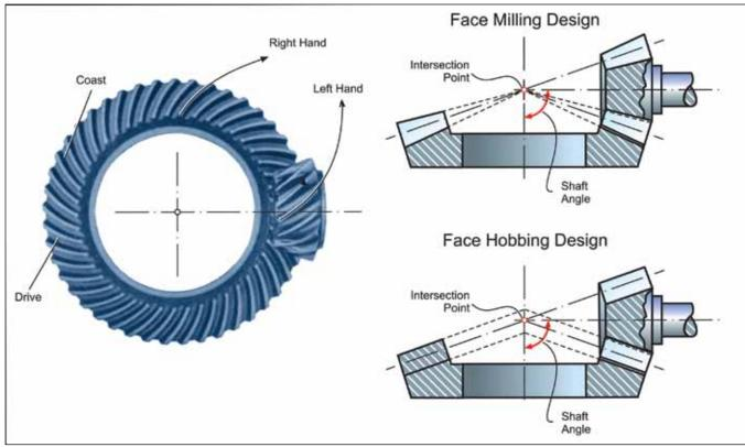
Figure 1—Spiral bevel gear geometry.
