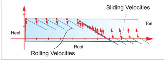
Figure 4—Rolling- and sliding-velocities of a spiral bevel gear set in path-of-contact points.
