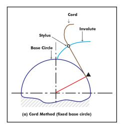
a fixed cylinder or circle (the base circle), as illustrated in Figure 1a. The involute path is traced by an imaginary point on the cord as it unwinds from the circumference of the base circle. Similarly, the involute can be generated by a rolling beam, as shown in Figure 1b. In this case, the involute is traced by an imaginary point at the end of the beam.
