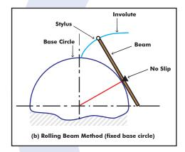
plan in which the involutes are traced is attached to the revolving base circle.
