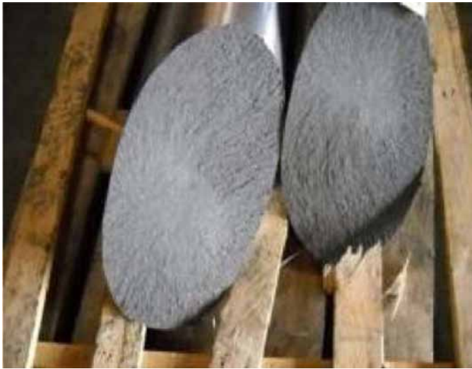
Figure 3—Sudden breakage due to hydrogen embrittlement.
