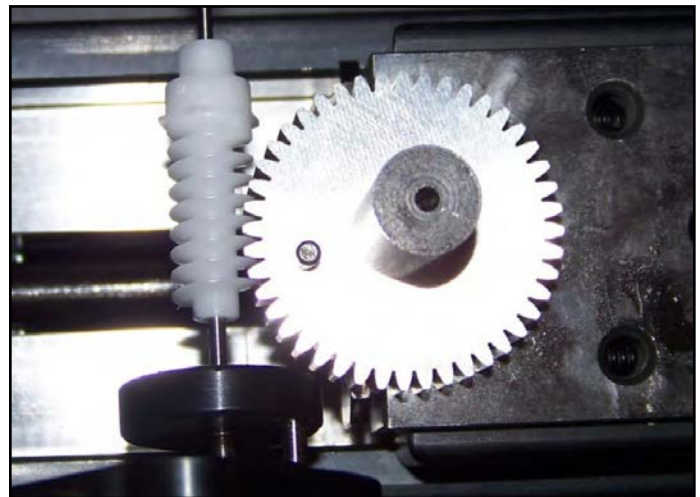
Figure 6 Plastic test worm in double-flank mesh with a master spur gear at an offset shaft angle (courtesy of Web Gear Services Ltd.).
