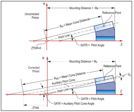
Figure 5 Principle of root angle correction.
