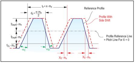
Figure 4 Pinion reference profile with positive profile side shift.
