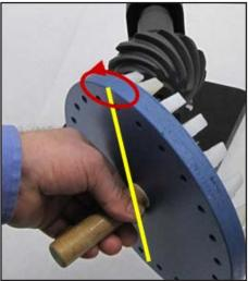
Figure 8 Cutter head tilt for the creation of generating crowning.
