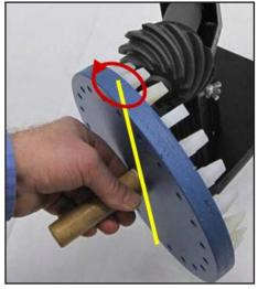
Figure 7 Cutter head tilt of a Formate pinion member.
