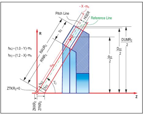
Figure 2 Impact of positive profile shift onto ring gear blank.
