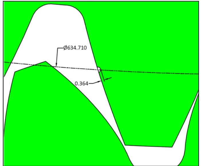
Figure 11 Detail of depth and position of pitting.
