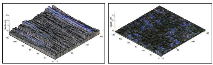
A machine surface finish (left) compared with an isotropic superfinish (right). Images courtesy of REM Surface Engineering.
