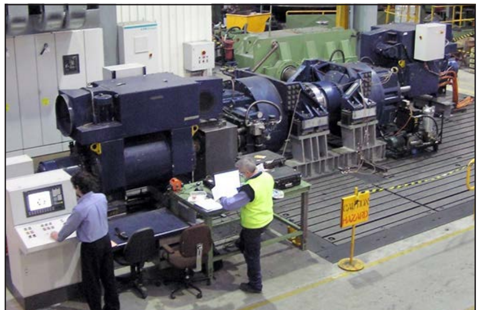
Figure 2 1MW-load GearTest installation at Hoffman Engineering, Perth, Australia.
