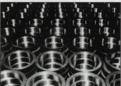
Fig. 26—Austempered steel, powdered metal sprag races.
