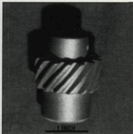
Fig. 22—AGI gear for timing on a light vehicle engine.
