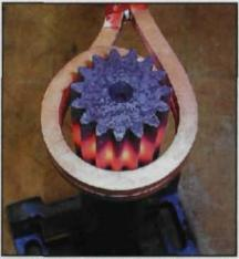
On a shaft, a spur gear pattern is induction hardened by a medium frequency and a high frequency transmitted at the same time via an induction hardening system from Electroheat Technologies L.L.C.
