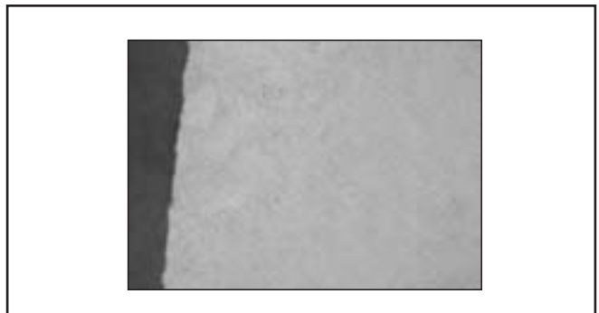
Figure 6—Gear microstructure (500X, 2% Nital)
