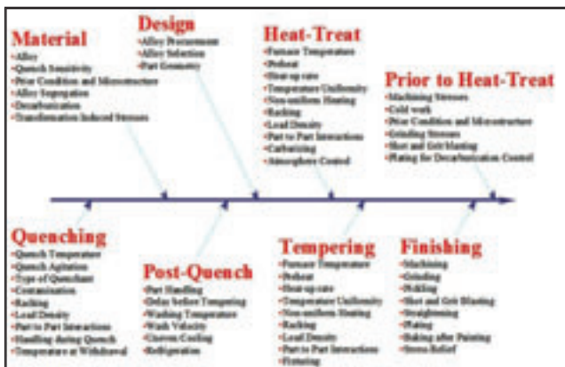
Figure 6—Fishbone diagram of the potential causes of residual stresses and distortion.
