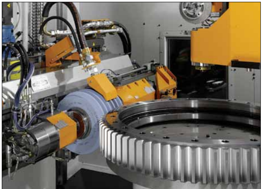
The LCS 1200 combines generating and profile grinding in one machine (courtesy of Liebherr).
