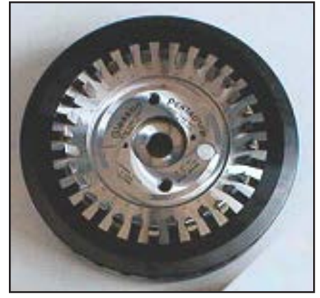
Figure 9 Fine-pitch Pentac face milling cutter head with large diameter.
