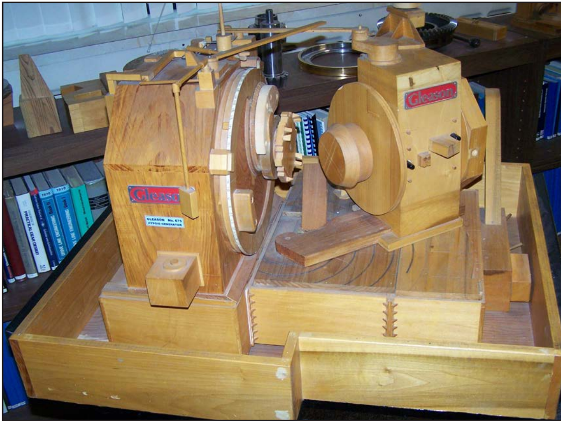
Figure 14 Wooden model of large cutting machine — Gleason No. 675.
