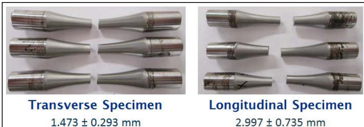
Figure 16 Images of typical transverse and longitudinal failed test specimens, illustrating the difference in axial failure location. The average axial distance of the fracture surface from the specimen mid-length (and corresponding standard deviation) are provided.
