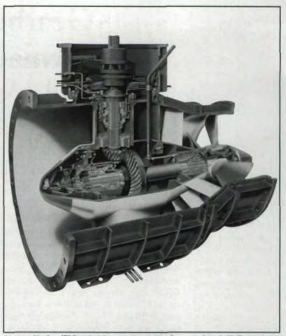
A water turbine from ATA Gears includes a set of its spiral beyel gears, as shown in this illustrated cross section. Entering the turbine, water turns the runner blades (right), driving the shafts and spiral bevel gears that gower the generator.
