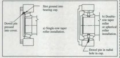
Figure 7-Common anti-rotation pin designs.
