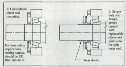
Figure 8—Seal designs for extended service life.
