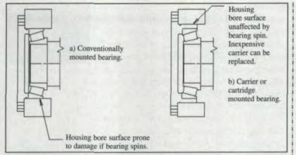
Figure 6-Bearing mounting for extended service life.
