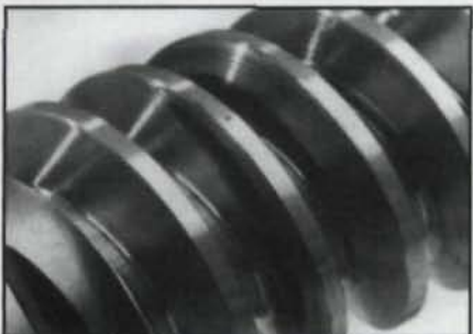
Fig. 3—Large score marks on a case-hardened worm.
