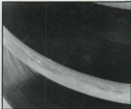
Fig. 10—Worm taken from test T1. Origin of the crack at the tip of the tooth.
