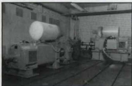
Fig. 2—Test stand for cracking damage, center distance a = 250 mm.
