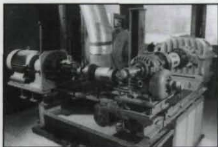
Fig. 1—Test stand for scoring damage, center distance a = 100 mm.
