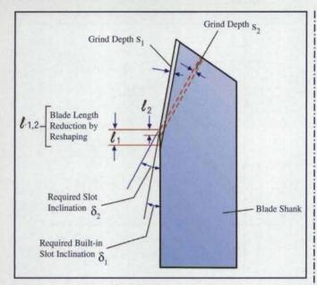
Figure 5—Blade length reduction after resharpening as a function of slot inclination.
