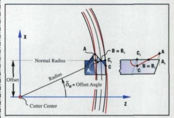
Figure 10—Relationship between hook angle and cycloidal path of different blade points.
