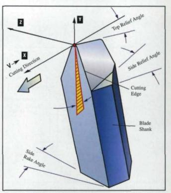
Figure 9—Pentac stick blade with permanent front face and pentagon-shaped cross section.
