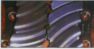
Figure 13—Left side-conventional, right side-cut with Spiroform cutter head.
