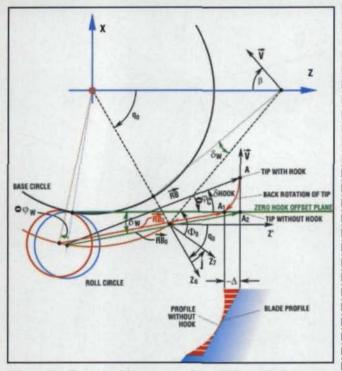
Figure 11—Epicyclical kinematics of two different blade types.
