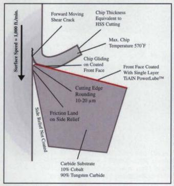
Figure 2-Chip forming mechanisms and specifications.
