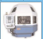
other ground parts. The machine's concept is to produce a complete workpiece by spreading the grinding operations over up to five different grinding stations on the same machine. The cycle time to produce a ground part is equal to the longest single operation plus transfer time.
