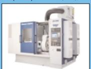
maximum tooth widths of 50 mm the Siemens CNC controller, enabling (1.97"), and module range of 0.5 to 4.5. The ZH 200 can combine its high cutting speeds with an optional, fast, fully integrated gantry loader system, thus offering the potential for significant improvements in overall cycle times.
