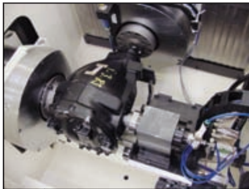
Figure 2—Typical mounting arrangement of bevel or hypoid housing on Oerlikon T60X.
