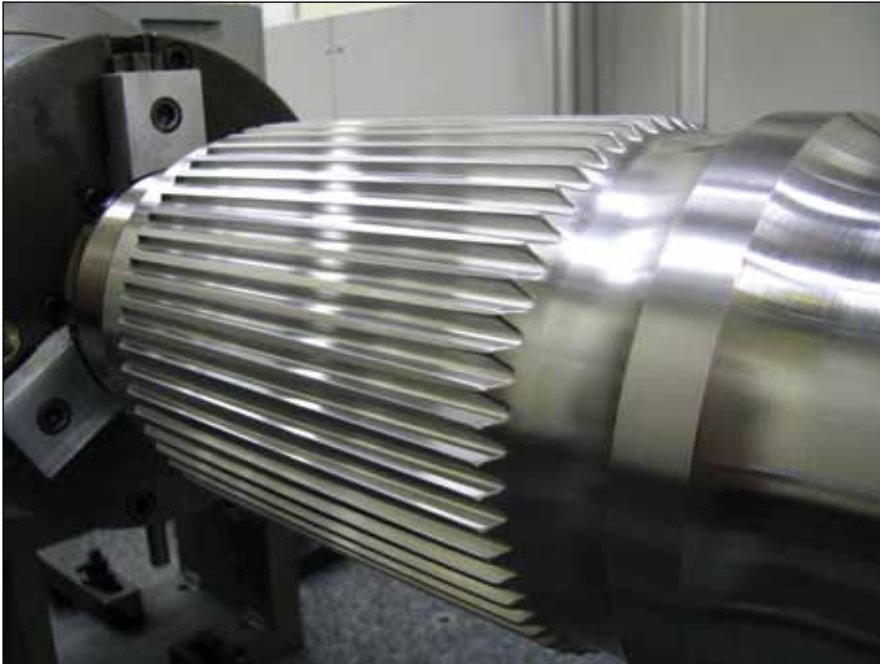
Gear measurements verified using Gear Pro software (courtesy of Carl Zeiss).
