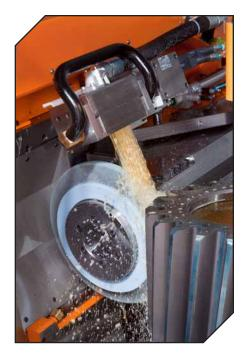
material for this wear-optimized grinding is no longer left to wear-out on the tip; as a result the risk of grinder-burn is minimized, and the workpiece is protected. Number of strokes and production time can be reduced as a result, depending on application.
