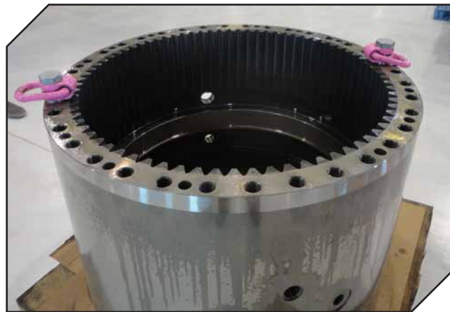
The large planetary component contained multiple internal gears of different geometry. In this view, the 12-module, 76-tooth, 282 mm face width gear geometry is shown. For semi-finishing this gear, Brevini Wind was able to use a duplex milling tool provided by Banyan Global Technologies for a previous ring gear application
