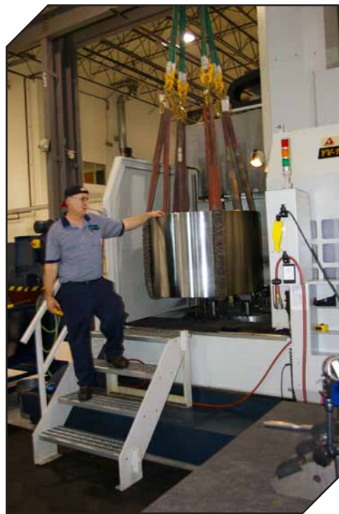
Machining Leader Tim Root removes one of the approximately 3,000 lb. planetary components from the Youji 1200 CNC vertical turning center, which Brevini Wind acquired and installed in the third quarter of 2012.
