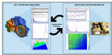
Figure 1 An integrated software solution for gear whine combining measured data capture and analysis with system-level simulations in a single environment with seamless data
