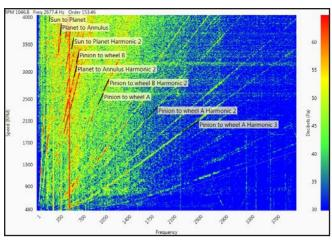
Figure 3 Measured noise displayed as a waterfall plot with excitation orders automatically labelled via data from a system simulation model.
