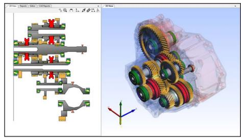
Figure 2 A system-level transmission simulation model.
