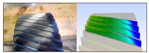
Figure 5 Measured and simulated loaded contact patterns.
