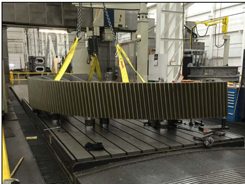
Figure 4 Prepping girth gear segment for reworking.
