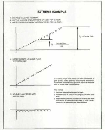
In summary, single flank testing can check all elements of gear quality, except possibly lead or spiral angle error, much faster and more thoroughly than individual elemental tests or double flank composite tests. This method:
