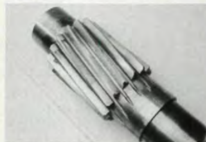
Fig. 6 - This new gear box failed because of misalignment even though it was supported between bearings.
