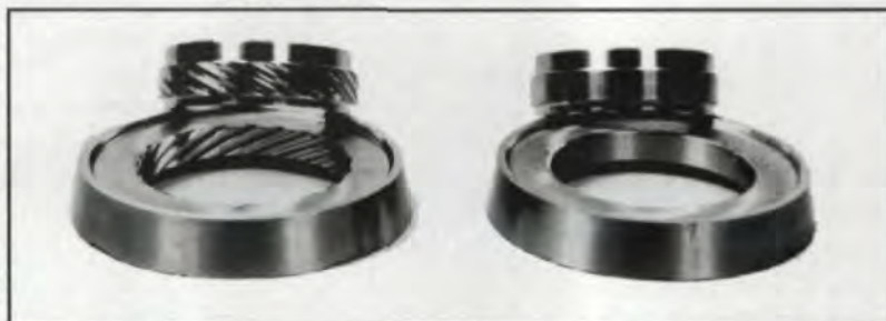
Fig. 6 — High helix angle internal and external gears ground from the solid with single layer, non-dressable CBN plated wheels.
