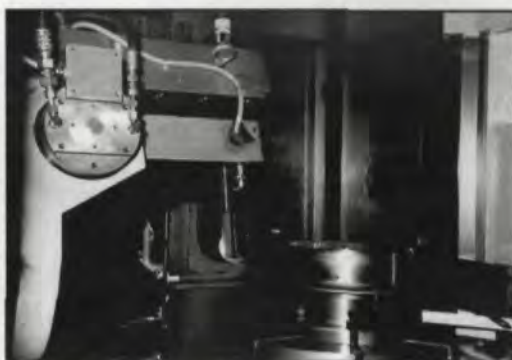
Fig. 5 — Pfauter CNC profile grinding machine with internal arm and single layer, non-dressable CBN wheel grinding a 124-tooth, 9.6 DP, 2.650 FW internal helical gear from the solid in 75 minutes.
