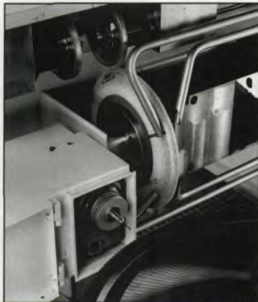
Fig. 10 — Integrated measuring probe on a Pfauter 1200 mm profile grinding machine grinding head. The probe is used to establish the angular position of the gear relative to the stock envelope condition on the workpiece and to inspect the finish ground gear.
