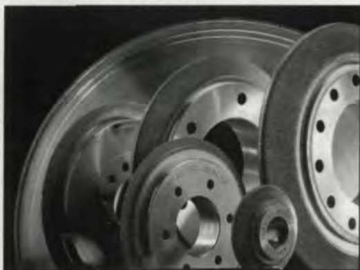
Fig. 11 — View of Pfauter-Winter CBN-plated wheels. The profile incorporated into the base body is defined by a CAD system which takes into consideration the quality of the profile to be achieved on the workpiece and the thickness of the layer of CBN crystal.
