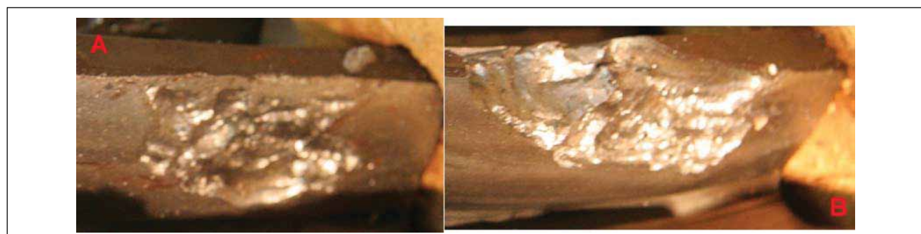
Figure 3—Heavy pitting often leads to local tooth fracture.
