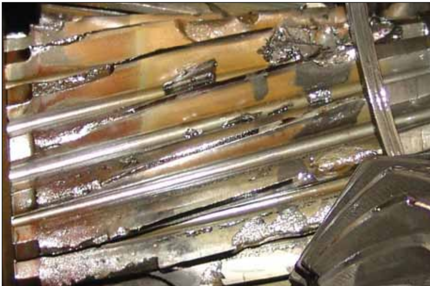
Figure 15—Partial tooth fractures resulting from spall crack progression.
